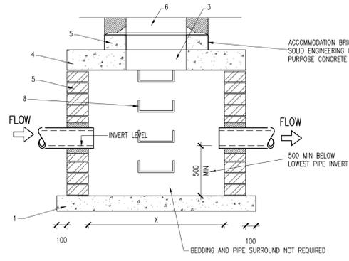
**CATCHPIT MANHOLE SECTION (FILTER DRAINS ONLY)**
